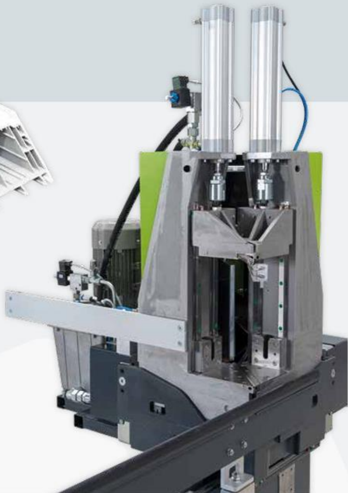
beheizte Messerkanten heated blade edges
